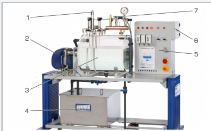
1 water level monitoring, 2 burner, 3 steam boiler model, 4 supply tank, 5 switch cabinet, 6 switch box for fault circuit, 7 pressure measurement equipment
